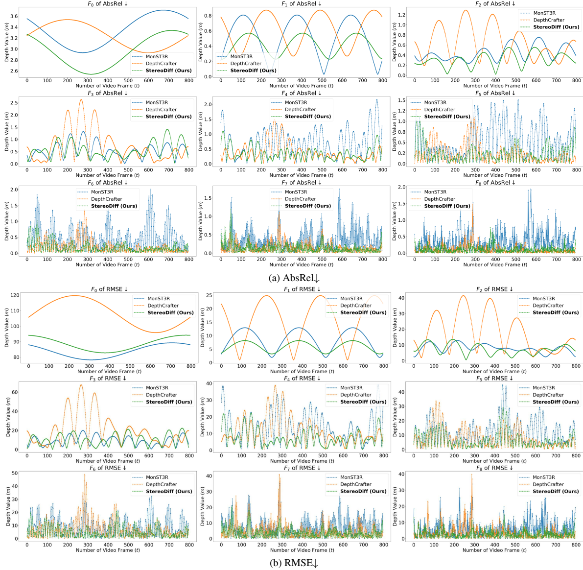
Figure 9. The error sequence of AbsRel↓ and RMSE↓ across different frequency domains on KITTI [19] dataset. Following Tab. 6, DFT and Inverse DFT are utilized to disentangle the components of the metric sequences into various frequency domains. Also for clearer visualization, only the modulus of the obtained complex numbers after Inverse DFT is plotted.
